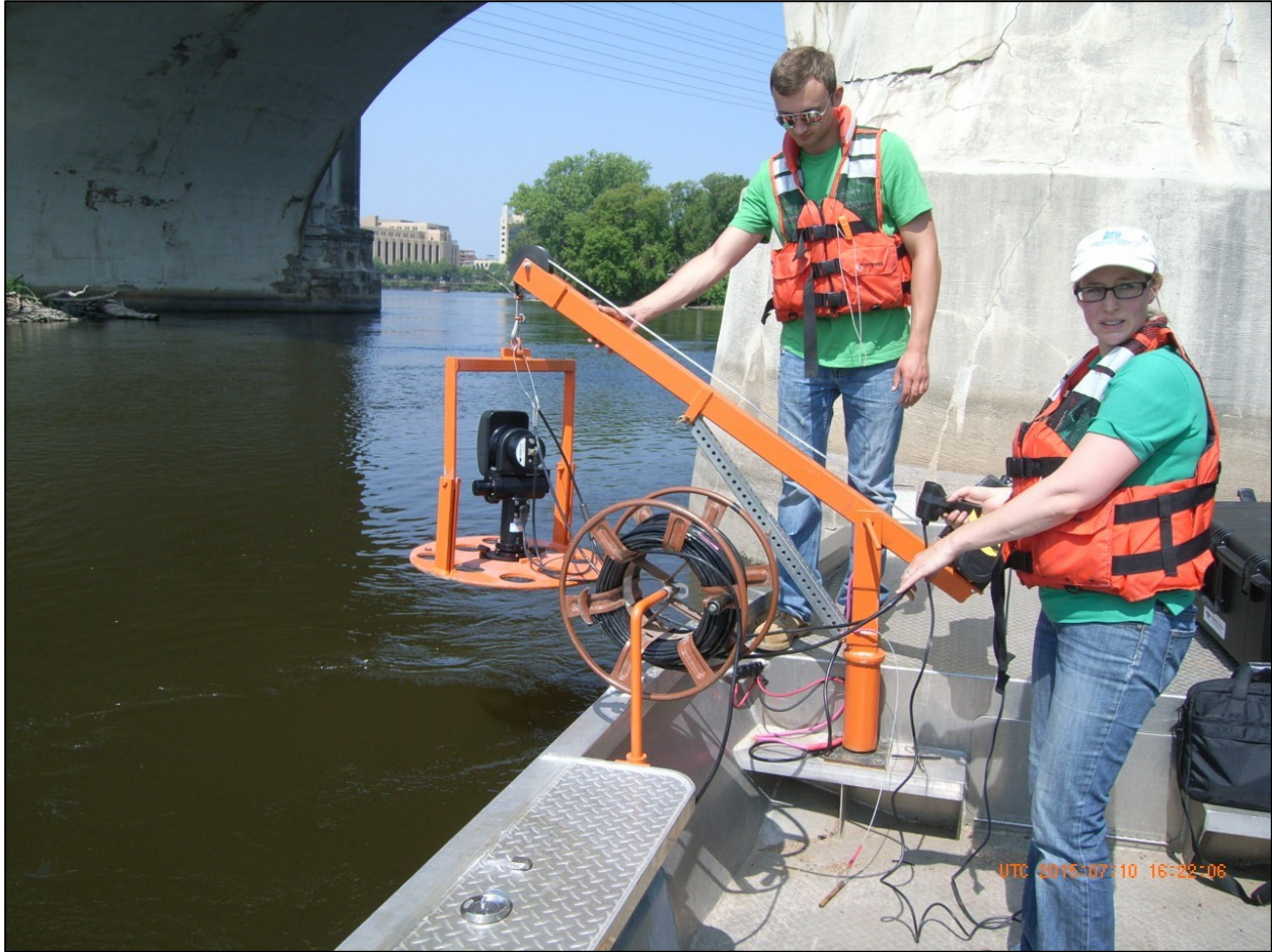
Figure 2-2: Metal Plate Stationary Deployment Method
