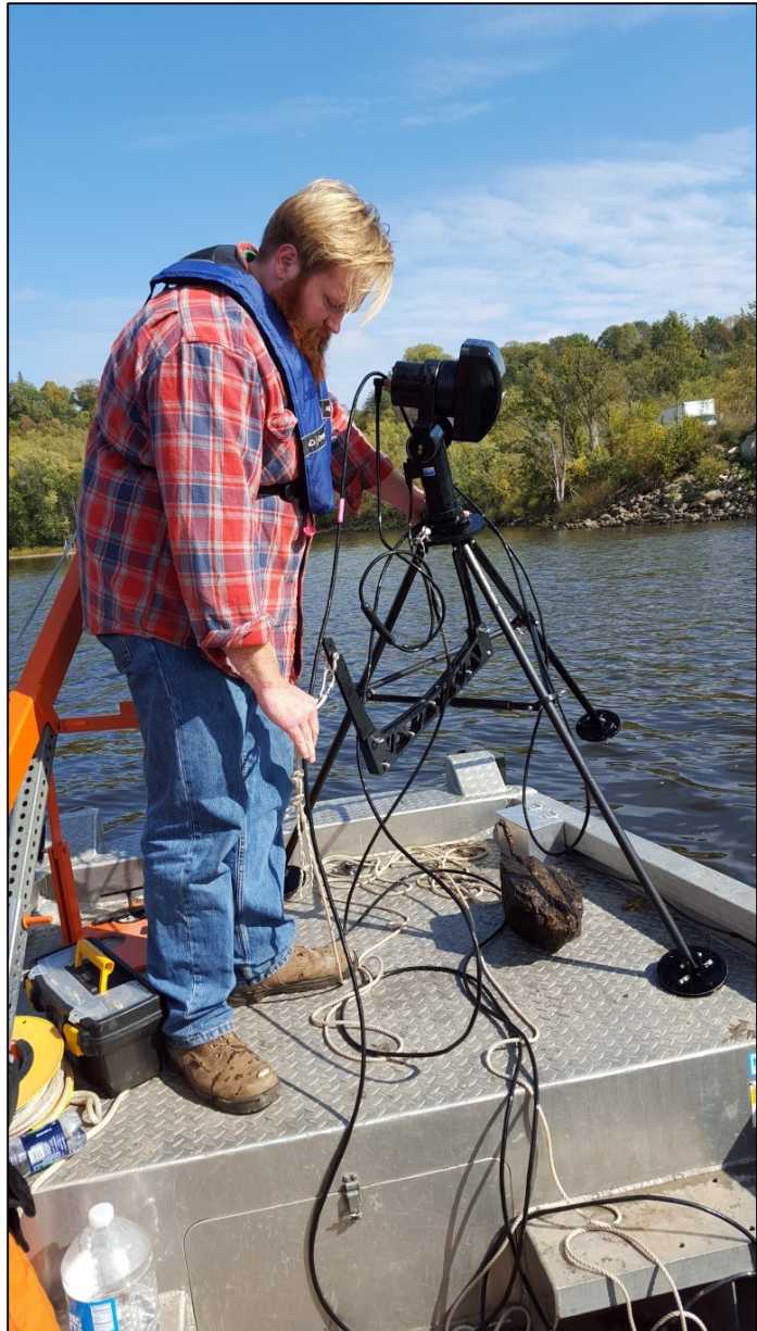
Figure 2-1: Tripod Stationary Deployment Method
