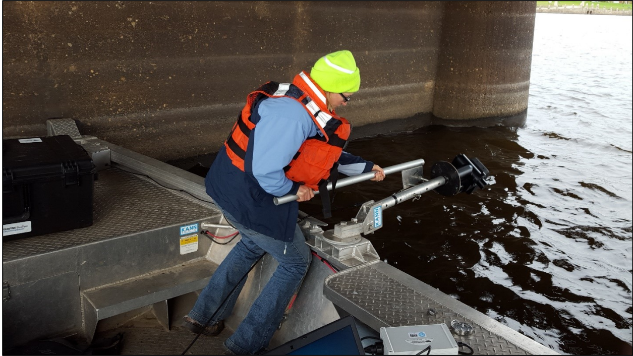
Figure 2-3: Boat Mounted Surface Stationary Deployment Method
