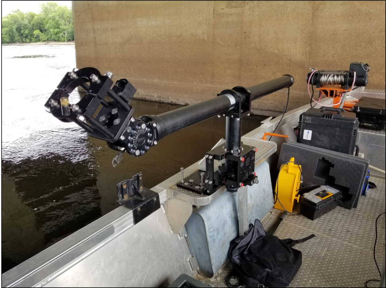
Figure 2-4: Boat Mount for Mobile Deployment Method
